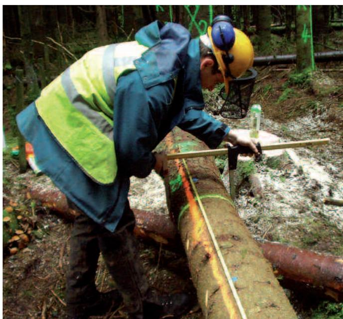
**Figure 3** Assessing the straightness of one of the standard logs (3.1 m).
